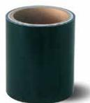
When attached to the surface of an object with unknown emissivity or a glossy object, this tape provides an emissivity of 0.95, enabling accurate non-contact temperature measurement. When using the tape, set the emissivity to  $\epsilon = 0.95$ . The tape is built with material resistant to heat up to 250°C (482°F).
