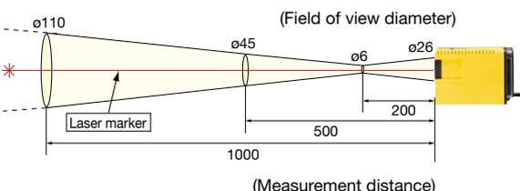
The laser marker points directly to the center of the field of view. The fields of view stated above are measurement diameters with an optical response of 90%. The size of the measurement target must be sufficiently larger than the figures shown in the above diagram.
